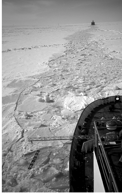
Figure 2: Photograph of typical conditions during our ship-based EM/laser measurements, taken from the bridge of DRANITSYN. ROSSIYA is leading (upper right), leaving behind a channel with broken ice. The EM system (lower left) is profiling only broken and disturbed ice. Note the scaffold boom construction which had to be built on the ship to suspend the instruments.
