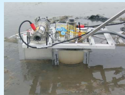
Fig. 4. Chamber deployment: Rhizon in situ sampler (RISS) combined with a benthic flux chamber.
