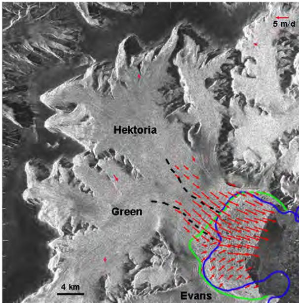
Fig. 5. Motion field of H-G-E glaciers derived from the ASAR IMS image pair, tr424, fr4941, IS2 HH, of 12 May 2004 and 16 June 2004 by means of amplitude correlation (blue line = grounding line, green line = ice front, black lines = flowlines of Green and Hektoria glaciers shown in Fig.6), superimposed to ASAR amplitude image of 12 May 2004.
