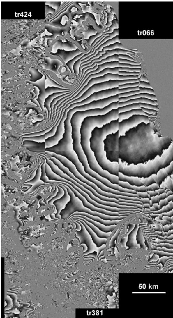
Fig. 9. ERS Tandem interferogram of Larsen C composed of track 424 (31 October – 1 November 1995), track 381 (28 – 29 October 1995) and track 066 (10 – 11 November 1995).
