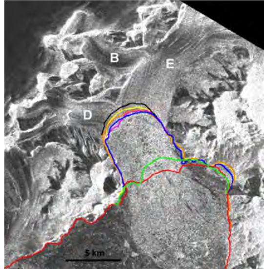
Fig. 3. ASAR IMS amplitude image, tr152, fr4941, IS2 HH, from 2 July 2004 showing ice front positions of Dinsmoor (D), Bombardier (B) and Edgeworth (E) glaciers (red = grounding line estimated from the ice edge in 1995, shortly after the ice shelf collapse, green = 01-11-1996, blue = 31-01-1999, yellow = 24-02-2002, black = 03-11-2002, orange = 04-04-2003, magenta = 13-02-2004).
