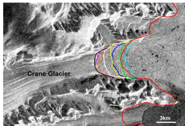
Fig. 7. ASAR IMS image, tr424, fr4959, IS2 HH, from 21 July 2004 showing ice front positions of Crane glacier (cyan = 23-04-2003, green = 24-12-2003, blue = 28-01-2004, yellow = 03-03-2004, white = 07-04-2004, orange = 12-05-2004, pink = 16-06-2004, black = 21-07-2004). The grounding line (red) is derived by ERS SAR interferometry.
