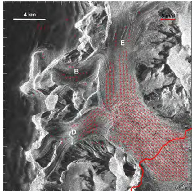
Fig. 4. Motion field of D-B-E glaciers derived from the ASAR IMS image pair of 28 May 2004 and 2 July 2004 by means of amplitude correlation (red line = grounding line), superimposed to ASAR amplitude image of 2 July 2004.
