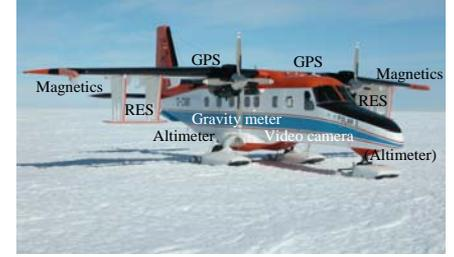
Fig. 2: Geophysical instrumentation on-board of POLAR2.
