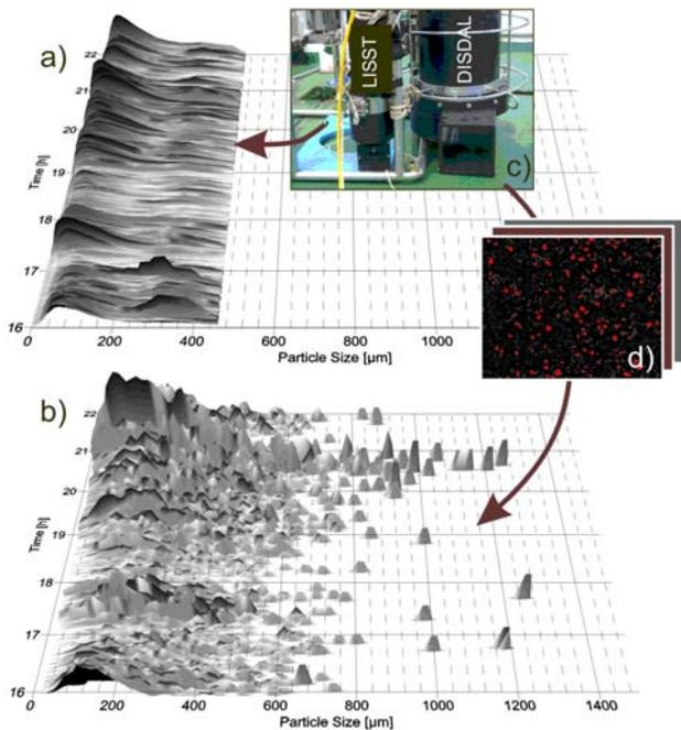
Figure 3. Temporal variation in absolute particle size distributions as derived from (a) LISST and (b) DISDAL in-situ photographs and image processing. The photos show (c) LISST and DISDAL mounted into an instrument frame and (d) a DISDAL image of SPM.
