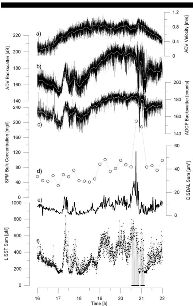
Figure 2. Time series of a) ADV current velocities, b) ADV backscatter intensity, c) ADCP backscatter intensity, d) Bulk concentration, e) DISDAL total particle area, and f) LISST total particle volume. The white lines show one minute running averages.
