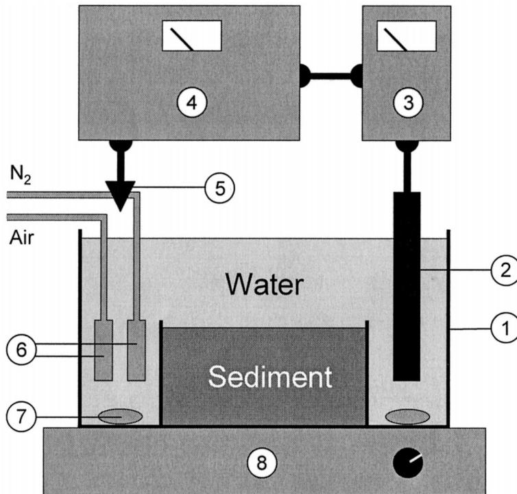
FIG. 1. Microcosms used for hypoxia experiments (side view). Numbered parts are acrylic aquarium (1), O<sub>2</sub> macroelectrode (2), oxymeter (3), O<sub>2</sub> control unit (4), magnetic valve (5), gas dispenser (6), stir bar (7), and magnetic stirrer (8).
