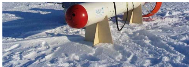
The EM-bird, a helicopter-towed electromagnetic sensor used for regional surveys of sea ice thickness (Photo: S. Goebell, Alfred Wegener Institute, Germany).
