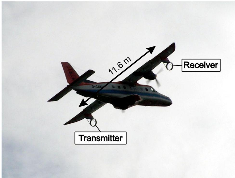
Figure 1. AWI Dornier 228 with the fixed wing sea ice thickness system
