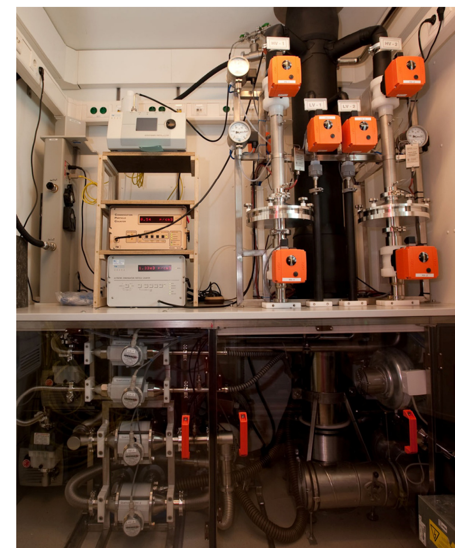
Fig. 2: High-volume aerosol sampling facility of Neumayer Station.
