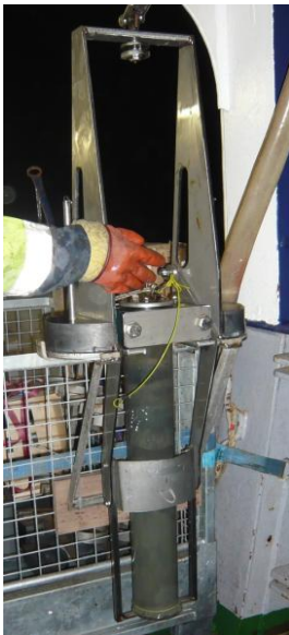
Fig. 5-6 The newly at IOW developed “Frahm Lot” short corer
