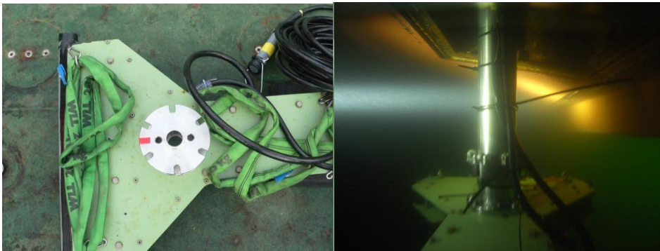
Fig. 5.1-1: (a) Mills-Cross transducer setup with housing plate on top and adapter flange for (b) subsurface installation
