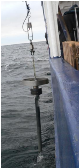
Fig. 5-5 „Rumohr“ type short corer (RL)
