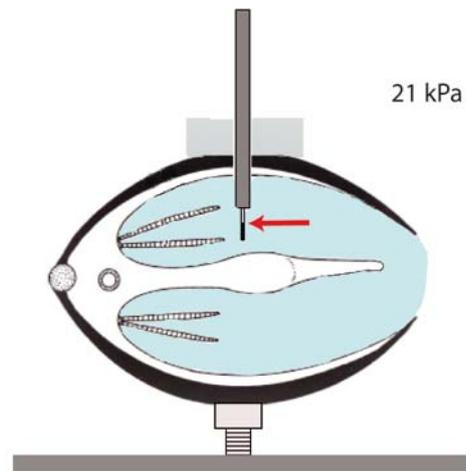
Fig. 2.3: Schematic overview of a fixed *Arctica islandica* in a laboratory aquarium at normoxic seawater ( $PO_2 = 21$  kPa), modified after Brusca and Brusca (1990). The implanted needle optode (red arrow) was inserted through a drilling hole in the shell and extended into the mantle cavity water (light blue) of the ocean quahog to measure the internal  $PO_2$ .
