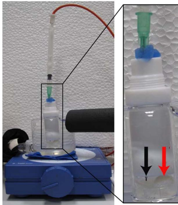
Fig. 2.5: Gill respiration measurement in *Arctica islandica* with an oxygen needle optode (black arrow), which is introduced into the cooled respiration chamber through a hole in the stopper. The gill sample (red arrow) is surrounded by 1.1 ml of respiration-buffer in the chamber.
