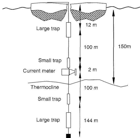
Fig. 44: Sediment trap array deployed under fast ice in the Drescher Inlet. Large traps were multitraps with 3 sample bottles each, set to switch every 6 days. Small traps had a single sample bottle. An Aanderaa current meter was placed above the pycnocline.
