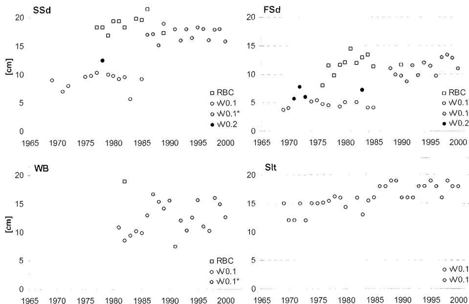
**Fig. 4.3.1:** Grab type and mean penetration depth per date as measured by depth of sediment contained in the grab. RBC: Reineck Box Corer 0.017m<sup>2</sup>; vV0.1: van-Veen grab 0.1m<sup>2</sup>; vV0.1\*: modified vV-grab 0.1m<sup>2</sup>; vV0.2: vV-grab 0.2m<sup>2</sup>.
