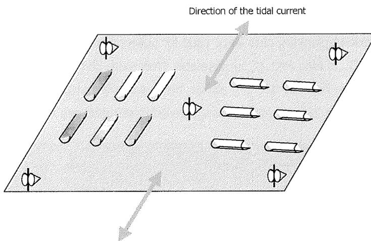
Figure 3. Experimental design. One set includes 12 grooves, 6 parallel and 6 perpendicular to the tidal current, and five plankton nets which direct themselves into the current.
