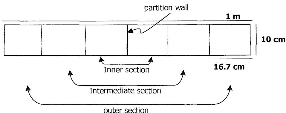
Figure 4. Grooves with partition wall in the middle and the six sections analyzed separately. Each section consists of 656 cm<sup>3</sup> of sediment.
