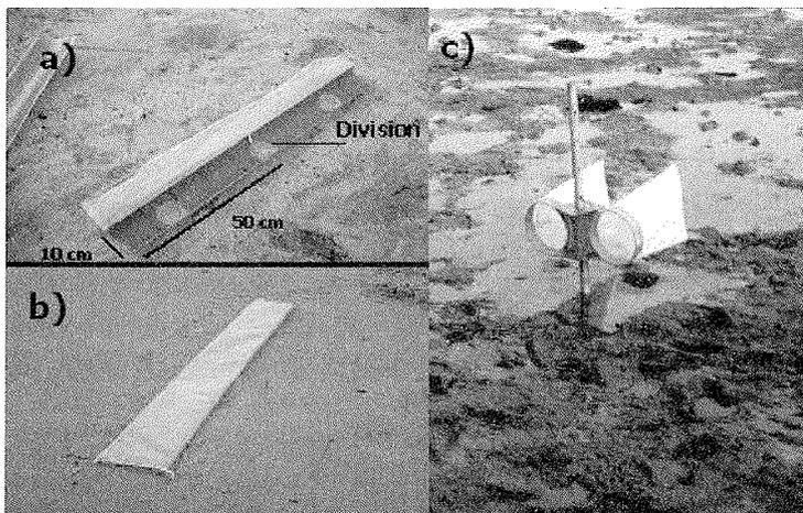
Figure. 2. Devices used: a) PVC grooves with middle division, b) position of a filled groove level with ambient sediment surface, c) plankton net to catch drifting organisms near the bottom in the tidal flow.
