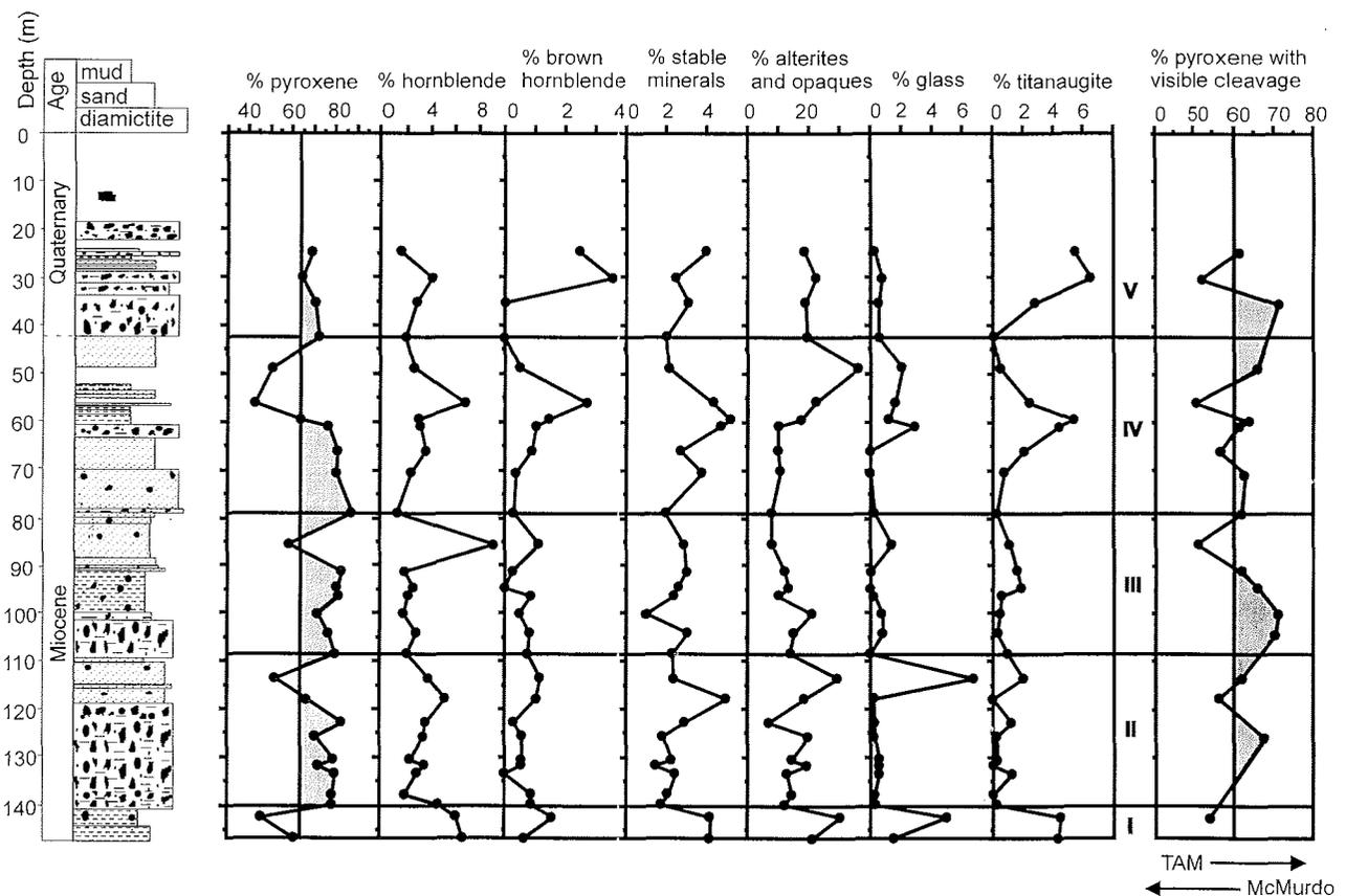
Fig. 2 - Percentage distribution of the main heavy mineral groups identified in the CRP-1 core. Five cycles can be observed (I - V). The column on the right-hand side indicates the percentage of pyroxenes with conspicuous cleavage which is indicative for a source in the Transantarctic Mountains (TAM), whereas pyroxenes with no cleavage indicate a likely volcanic source in the region of the present-day Ross Ice Shelf.
