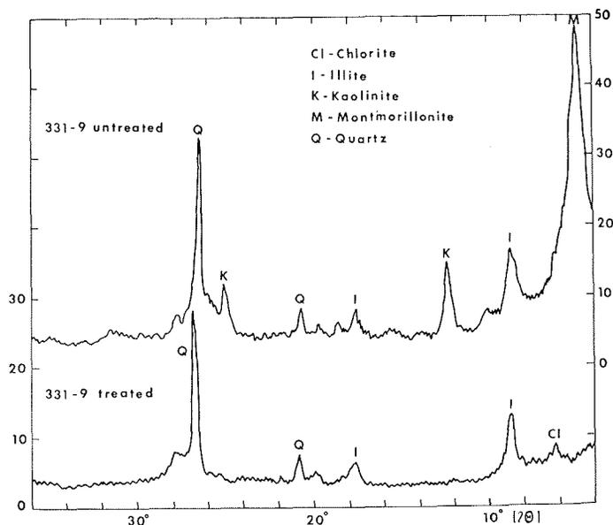
Fig. 4: X-ray diffractograms of the clay mineral assemblage, band 9, core no. 331.
