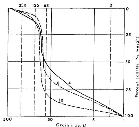
Fig. 3: Grain size distribution for selected bands, core no. 331.
