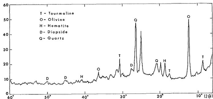
Fig. 5: Typical x-ray diffractogram of the heavy mineral assemblage, core no. 331.
