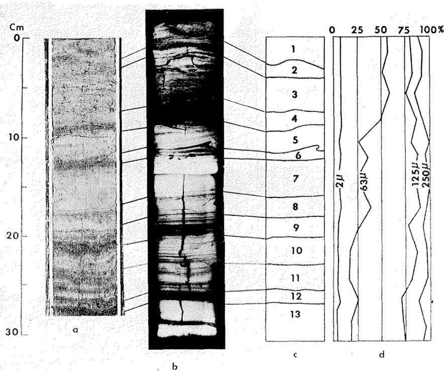
Fig. 2: Core no. 331. a. photograph, b. radiograph, c. band numbers, and d. grain size distribution.
