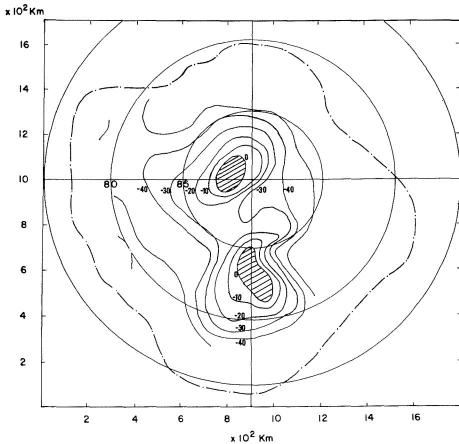
Fig. 15: Basal isotherms ( $T_b$  °C) constructed from Figs. 6 (Z) and 13 (T<sub>b</sub>) with  $T_b = T_s + \gamma_s Z$  and  $\gamma_s = 30$  °C km<sup>-1</sup>. The hatched areas have the pressure-melting temperature  $T_p = -0.77 Z$  °C (Z in km).
