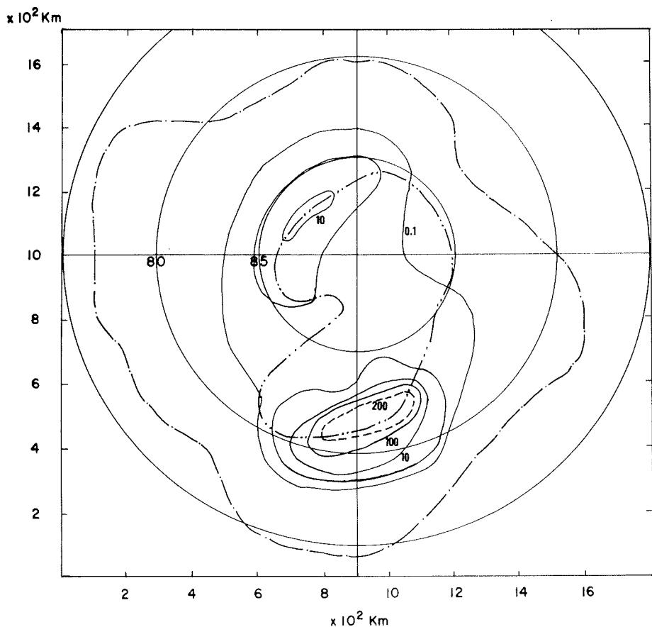
Fig. 8: Volume flux  $\bar{V}Z$  ( $m^3/m\text{ a}$ ). The line ... separates the regions with surface accumulation and surface ablation (cf. Fig. 9).
