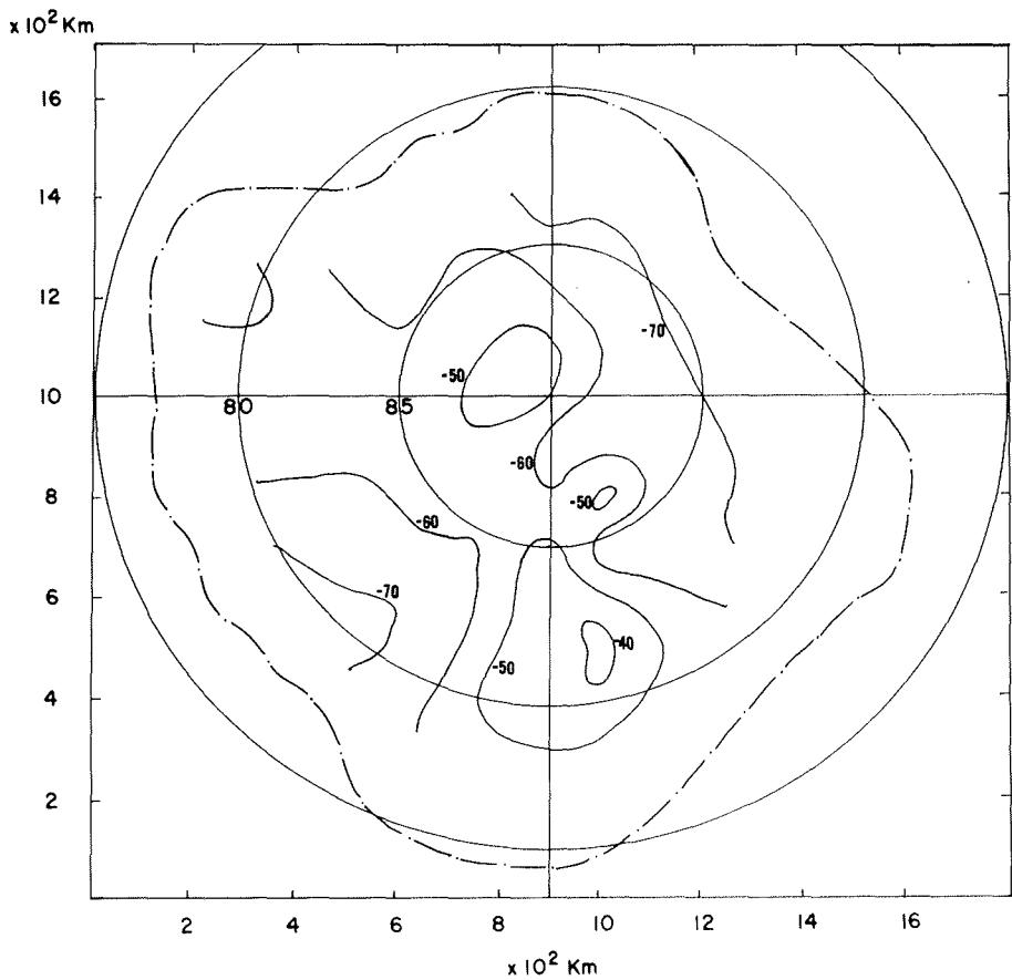
Fig. 14: Basal temperature ( $T_b$ , °C) constructed from Figs. 6 (Z) and 13 ( $T_s$ ) with  $T_b = T_s + \gamma_e Z$  and  $\gamma_e = 15^\circ \text{C km}^{-1}$ .
