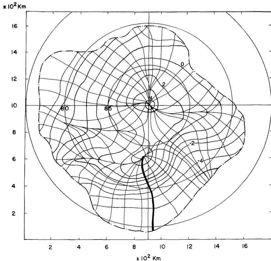
**Fig. 3:** Surface elevation (km) contours (redrawn from a digitization of the contours in Fig. 1) of the north polar ice cap, and orthogonal ice flowlines. The heavy line marks the cross section of Figs. 11 and 12.
