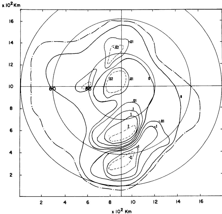
Fig. 9: Isotachs ( $\text{mm a}^{-1}$ ) of the vertical velocity at the ice cap surface. These velocities equal the divergence of the volume flux (Fig. 8) and, in steady-state conditions, the rates of accumulation ( $>0$ ) and ablation ( $<0$ ).
