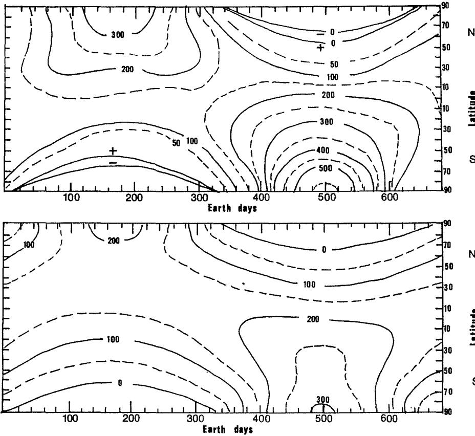
Fig. 16: Daily radiation intake ( $\text{W m}^{-2}$ ) of different latitudes during a Mars year. Bottom: Insolation for the present obliquity  $\epsilon = 25^\circ$ . Top: Increase in insolation for  $\epsilon = 35^\circ$ .
