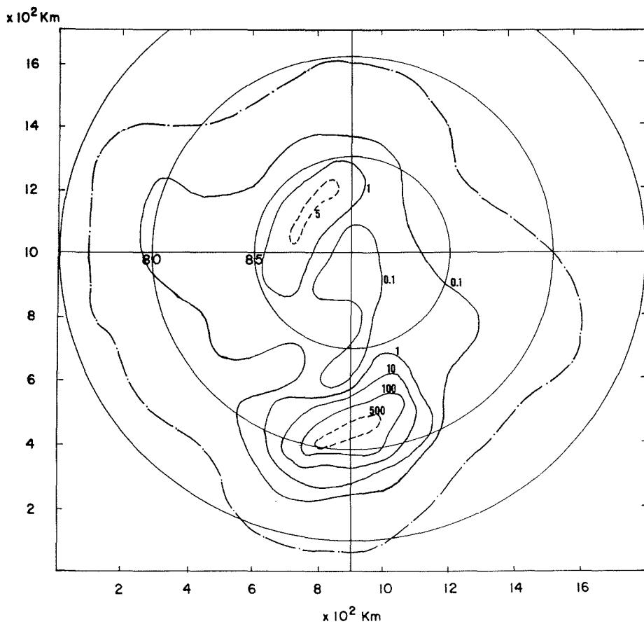
**Fig. 7:** Isotachs ( $\text{mm a}^{-1}$ ) of the horizontal ice velocity averaged over depth  $\bar{V} = k(T)\tau_5 Z$ . For explanation see text.
