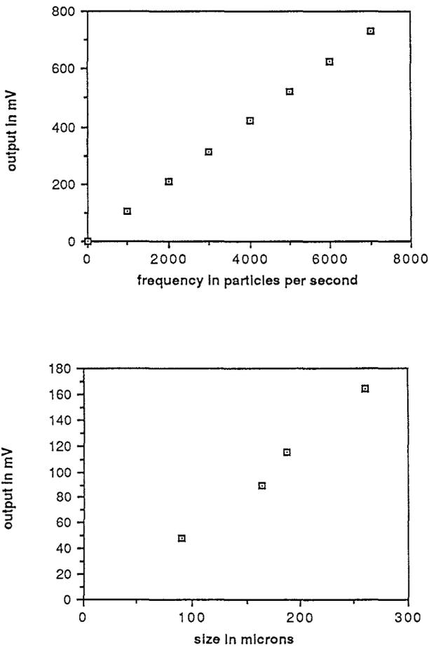
Fig. 2: Calibration curves for frequency and size of snow particles.
