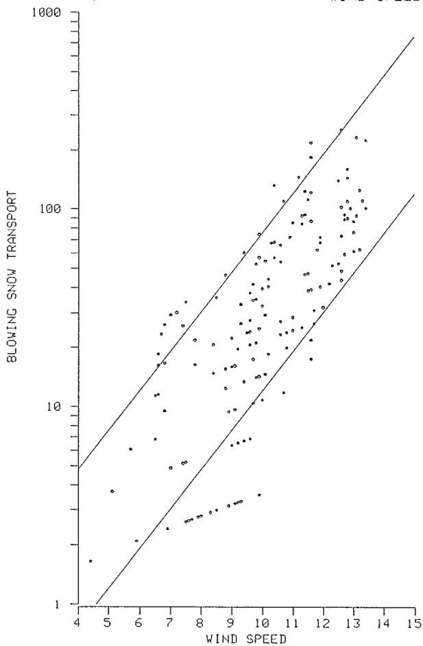
Fig. 7: Total flux of drifting snow ( $\text{g m}^{-1} \text{s}^{-1}$ ) against wind speed ( $\text{m s}^{-1}$ ) as observed in 1982, South Pole station. The two lines represent values from traditional snow traps as summarized by KOBAYASHI (1978).
