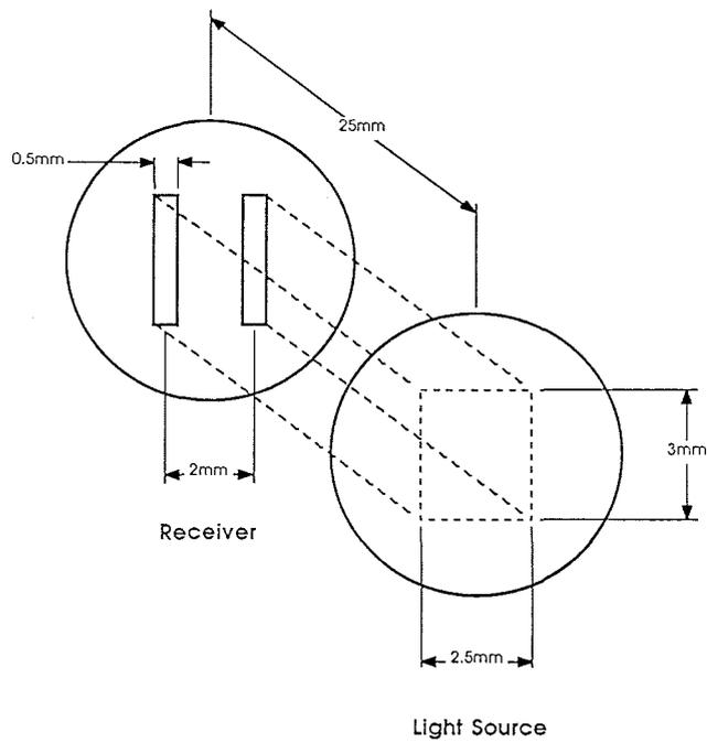
Fig. 1b: Schematic diagram of snow particle counter.
