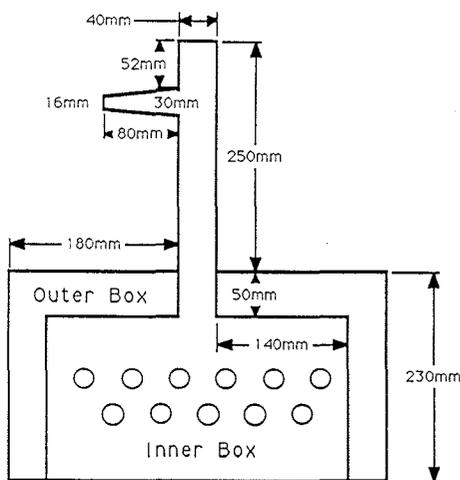
Fig. 3: Schematic diagram of conventional snow trap used in an inter-comparison.
