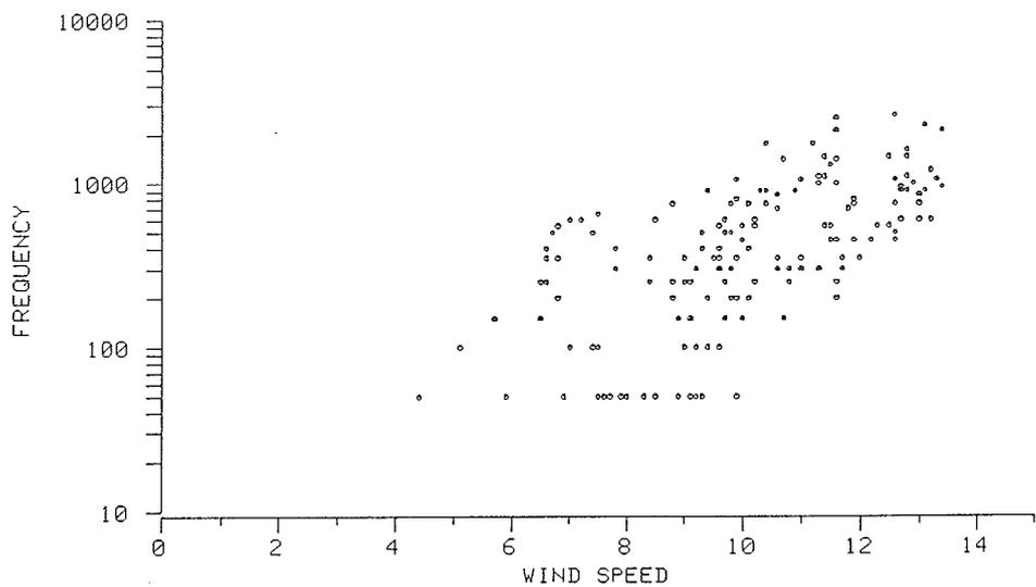
Fig. 6: Frequency (particles  $\text{cm}^{-2} \text{s}^{-1}$ ) against wind speed ( $\text{m s}^{-1}$ ), all events of 1982, South Pole station.
