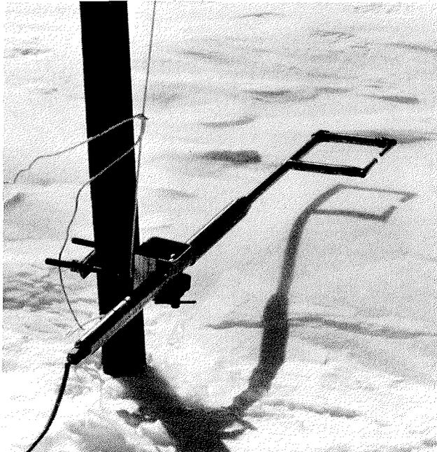
Fig. 1a: Photo of snow particle counter and its schematic function.
