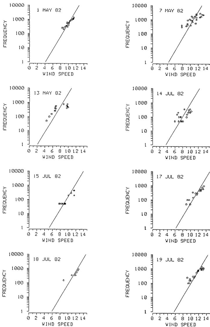
Fig. 5: Frequency (particles  $\text{cm}^{-3}\text{s}^{-1}$ ) against wind speed ( $\text{m s}^{-1}$ ) for eight separate events in 1982, South Pole.
