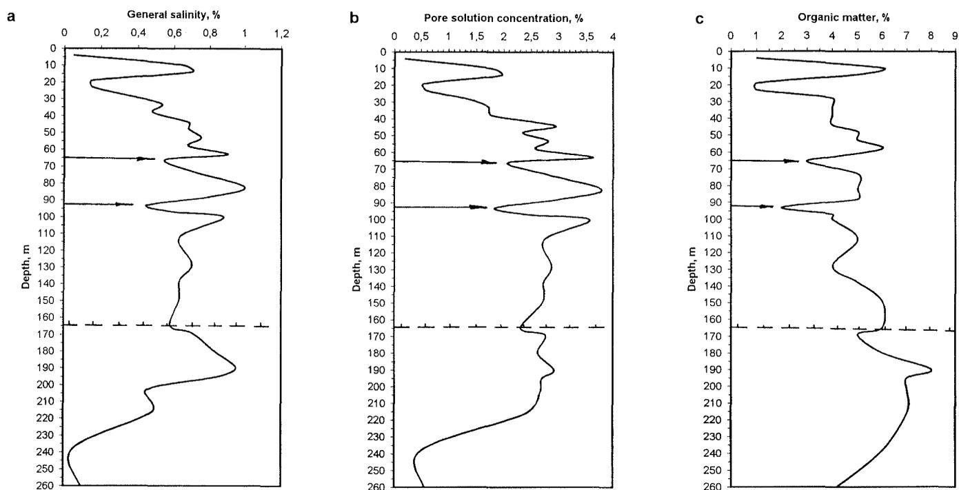
**Fig. 5:** Gas release in relation to (a) general salinity, (b) pore solution concentration, and (c) organic matter content according to monitoring well 610-P-2 drill cores. Gas releasing intervals at depths of 63-67 m (gas flow rates 500 m<sup>3</sup>/day) and 91-95 m (gas flow rates 1000 m<sup>3</sup>/day); freezing front at approx. 165 m.
