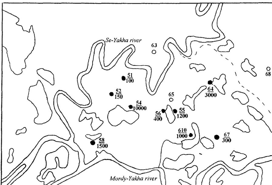
Fig. 4: Map showing locations of monitoring wells. Open circles = well cluster number; filled circles = wells producing from depth interval 60-120m and maximum gas flow rate (m³/day).
