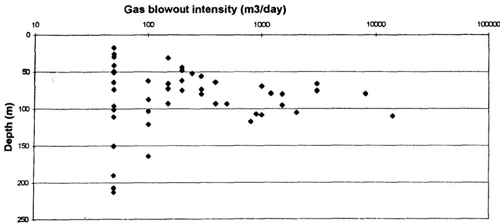
Fig. 3: Distribution of gas blowouts and their intensities with permafrost depth at Bovankovo gas field; generalized data from 40 wells.
