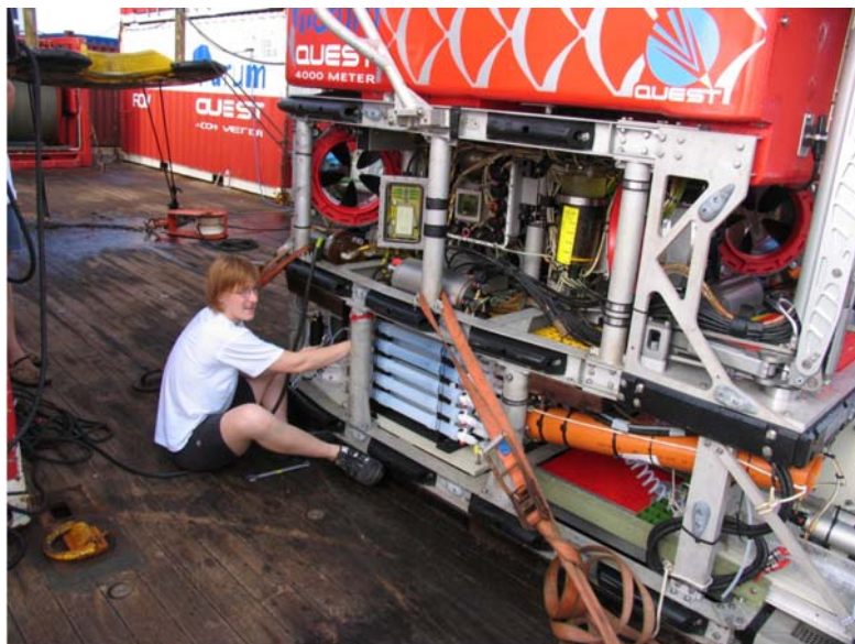
Fig. 1.5: The fluid sampling system “KIPS” mounted on the starboard back side of the Bremen MARUM ROV (“Quest”) tool sled
