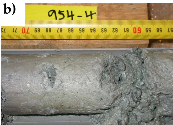
Fig. 2.10.: Selected core photographs showing a) the heterogeneity of rock type recovered during a single drill hole (957RD) located north of the Irina II mound. b) mineralized core sections (counterclockwise from upper left). Clay-rich material with abundant serpentinized rock fragments next to a smoking crater. Sulfide pebbles within altered host rock (core 962). Sulfide-impregnated serpentinite sand (core 954). Fe-oxyhydroxide bearing sediment and semi-lithified sediment recovered from east of the main hydrothermal area (core 959).
