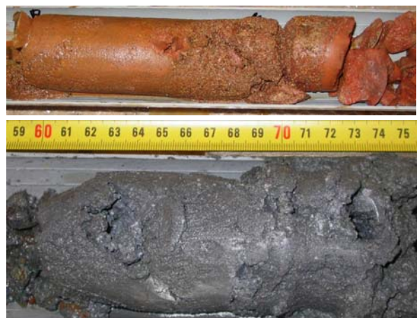
Fig. 2.10.: Selected core photographs showing a) the heterogeneity of rock type recovered during a single drill hole (957RD) located north of the Irina II mound. b) mineralized core sections (counterclockwise from upper left). Clay-rich material with abundant serpentinized rock fragments next to a smoking crater. Sulfide pebbles within altered host rock (core 962). Sulfide-impregnated serpentinite sand (core 954). Fe-oxyhydroxide bearing sediment and semi-lithified sediment recovered from east of the main hydrothermal area (core 959).
