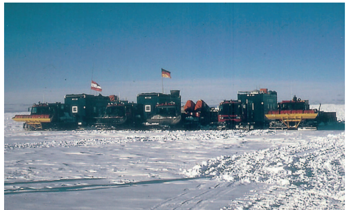
Fig. 1: Heavy logistical equipment with tractors (Pistenbullis) and freight sledges with mounted living containers was the preferred transportation mode during the expeditions 1985/86 and 1989/90. Here, the traverse at the start from Georg von Neumayer Station in December 1985.
