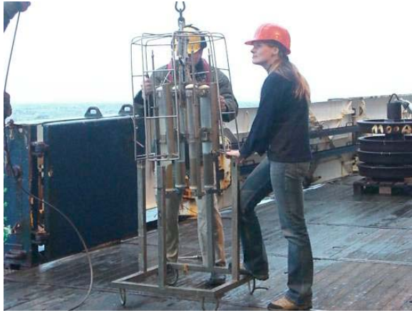
Fig. 3.28: Minicorer deployment during ANT-XXIV/3
