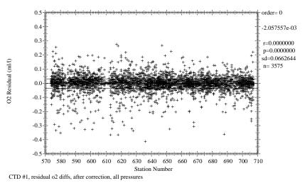
Figure 8.4.0 I4/I5W/I7C O2 residual differences vs station # (after correction).
