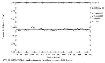
Figure 8.3.1 I4/I5W/I7C CTD #1 preliminary conductivity offsets by station number.
