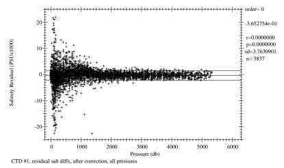
Figure 8.3.5 I4/I5W/I7C Salinity residual differences vs pressure (after correction).
