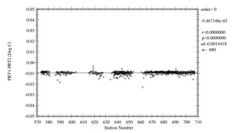
Figure 8.2.0 I4/I5W/I7C Shipboard comparison of CTD #1 primary/secondary PRT temperatures, pressure > 2000 db.
