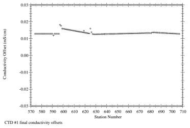
Figure 8.3.4 I4/I5W/I7C CTD #1 conductivity offsets by station number.
