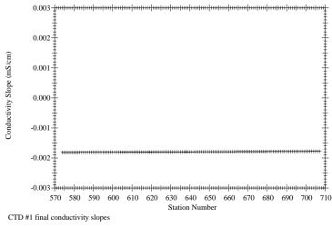
Figure 8.3.3 I4/I5W/I7C CTD #1 conductivity slope corrections by station number.
