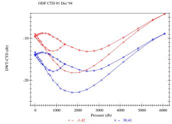
Figure 7.0 Pressure calibration for ODF CTD #1, December 1994.
