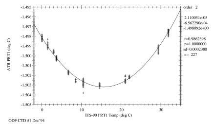
Figure 7.2 Primary PRT Temperature Calibration for ODF CTD #1, December 1994.
