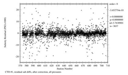
Figure 8.3.6 I4/I5W/I7C Salinity residual differences vs station # (after correction).
