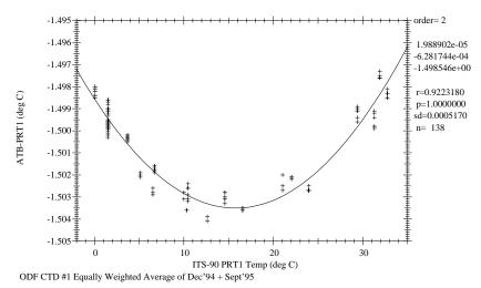
Figure 8.2.1 WOCE95 Primary temperature correction for ODF CTD #1, Dec.94/Sept.95 equally weighted average.
