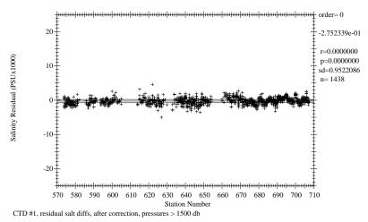
Figure 8.3.7 I4/I5W/I7C Deep salinity residual differences vs station # (after correction).
