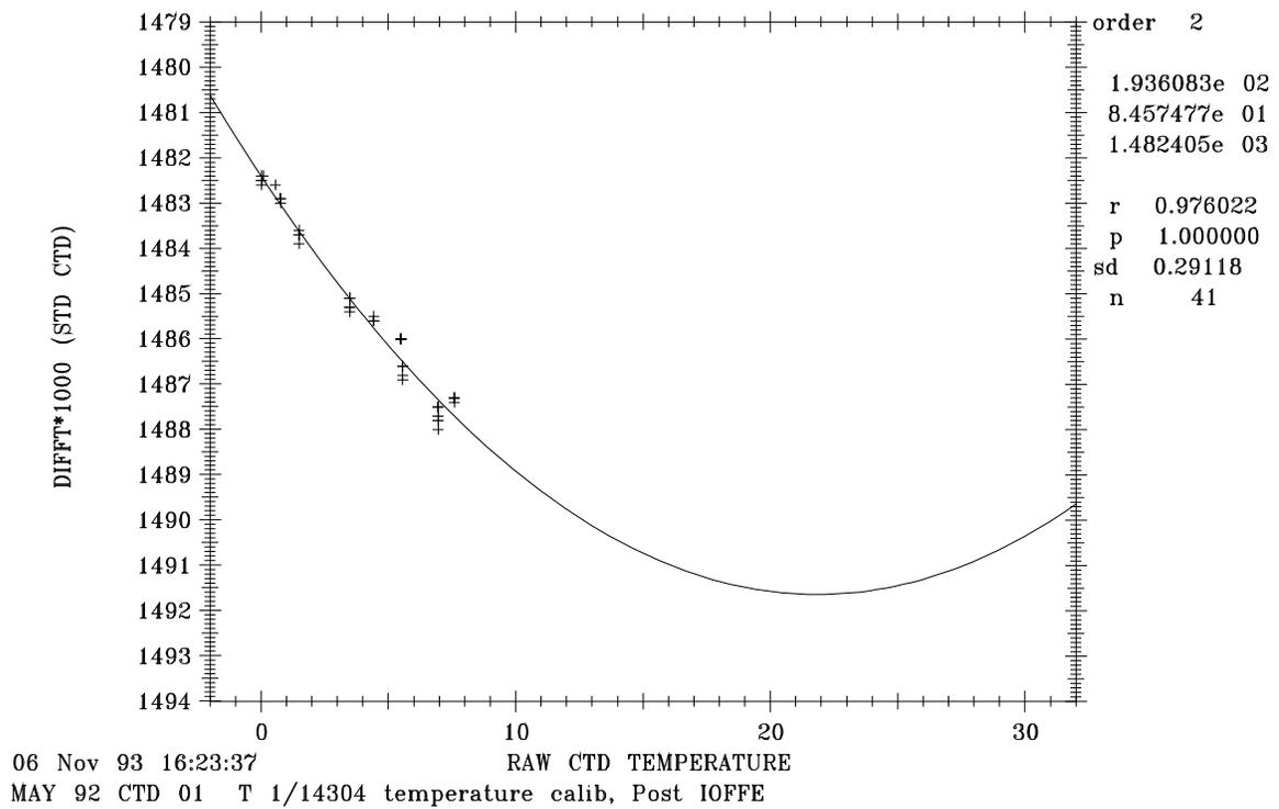
Figure 2b: CTD #1 Post-cruise PRT-1 Temperature Calibration
