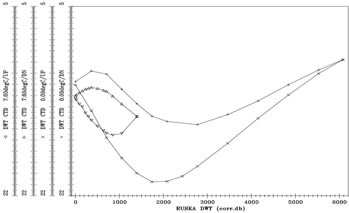
Figure 1b: CTD #1 Post-cruise Pressure Calibration
