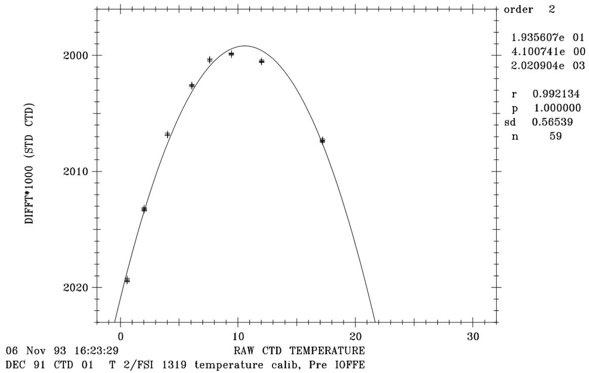
Figure 3a: CTD #1 Pre-cruise PRT-2 Temperature Calibration
