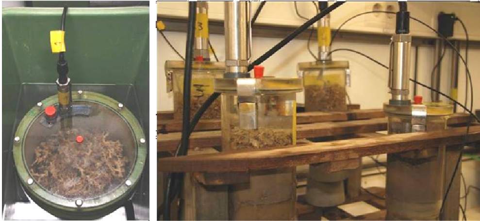
Fig. 6. Left-hand panel: Incubated coral rubble with associated epifauna. Right-hand panel: incubated cores in core holder, presens optode and temperature recorder is in core in the RH corner.
