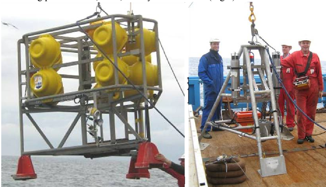
Fig. 7. Left-hand panel: the NIOZ lander used for baited experiment. Right-hand panel: the OceanLabsystem with the ballast and bait in the foreground.
