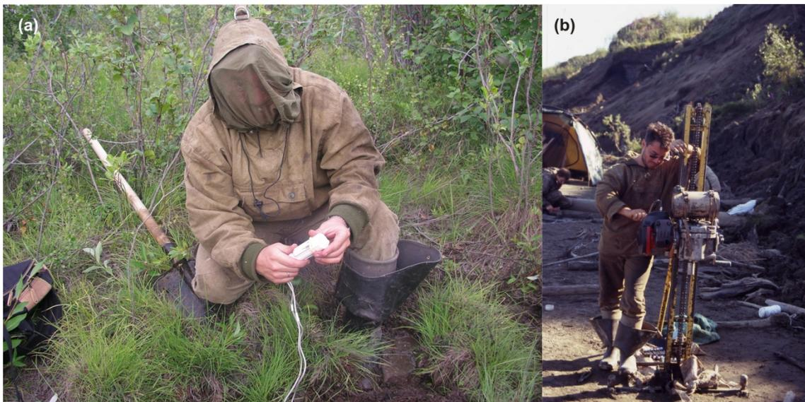
**Figure 3-1:** Impressions from the drilling work: (a) logger installation at borehole 2-08; (b) the rotary drilling equipment UKB-12/25 in use at borehole 3-08.
