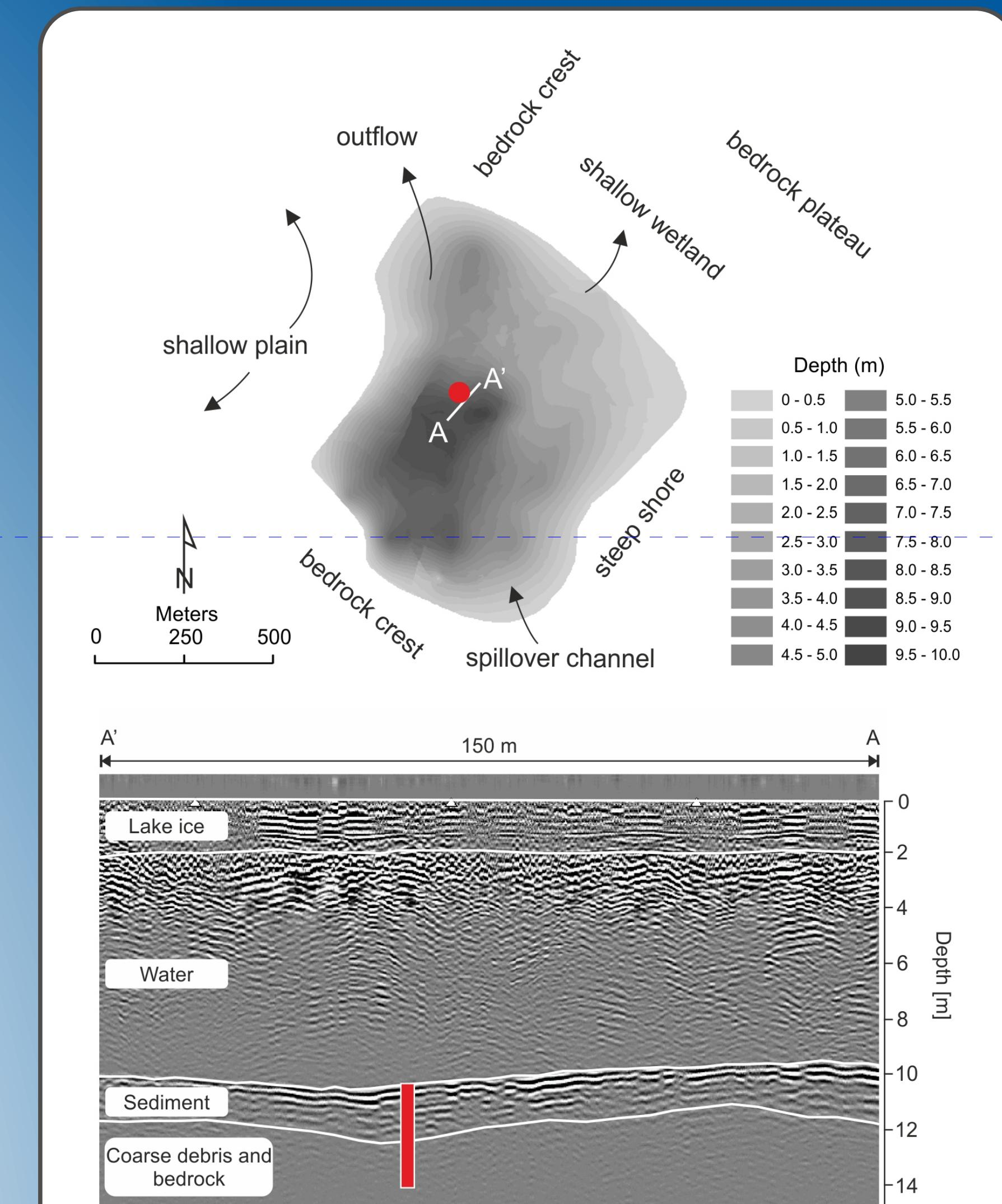
Trout Lake bathymetry and coring location (red circle) in April 2009. The bathymetry map is based on echosoundings and depths extracted from ground penetrating radar (GPR) tracks collected on the lake ice. Interpreted GPR profile (100 MHz) across the coring location (red bar).
