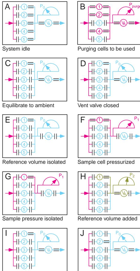
Figure 2—2 Operating sequence of the Quantachrome penta-pycnometer. Blue lines and cells are under ambient pressure  $P_a$  ( $P_a = P_0$ ). Red lines and cells are
