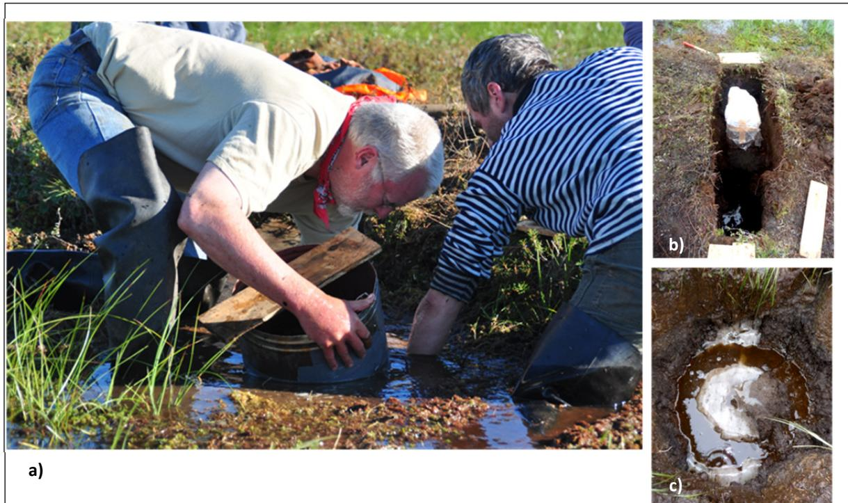
**Fig. 6-8:** Collection of the peat profiles. a) Getting out the peat profile LHC-11 j20,20 with the tube corer. b) Ditch to get the three ridge peat profiles. In the middle of the ditch is the covered peat profile LHC-11 j18,80 visible. c) Ice wedge under the profile LHC-11 j14,30 in the central depression.
