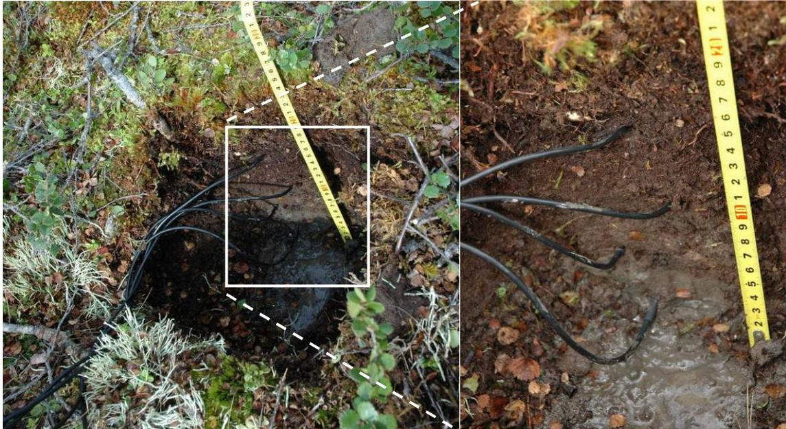
**Fig. 3-7:** Installing ground temperature data loggers in the polygonal wall. They were installed shifted against one other with approx. 5 cm height distance between each sensor. We installed the lowest one directly above the permafrost table on July 19<sup>th</sup>.
