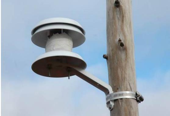
**Fig. 3-5:** Air temperature data logger at the pole in 2 m height with a solar radiation shield.
