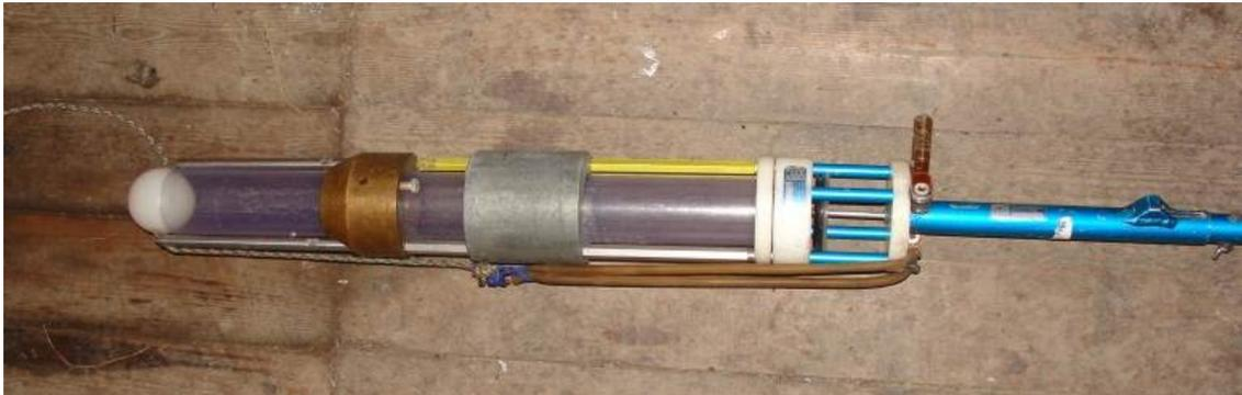
**Fig. 5-3:** UWITEC gravity corer
