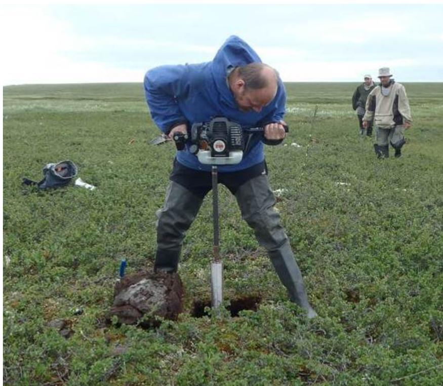
**Fig. 9-1:** Drilling of the borehole 11KH-1907-1 in the upper alas level.
