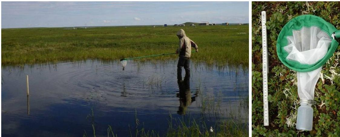
**Fig. 3-10:** Sampling with the plankton net (20 cm in diameter, mesh size of 65  $\mu$ l). The 100ml PE-bottle was used for plankton samples only, we caught ostracods and macrozoobenthos with a similar net without PE-bottle.
