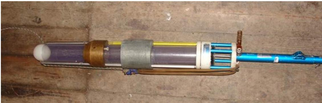
Fig. 5-3: UWITEC gravity corer
