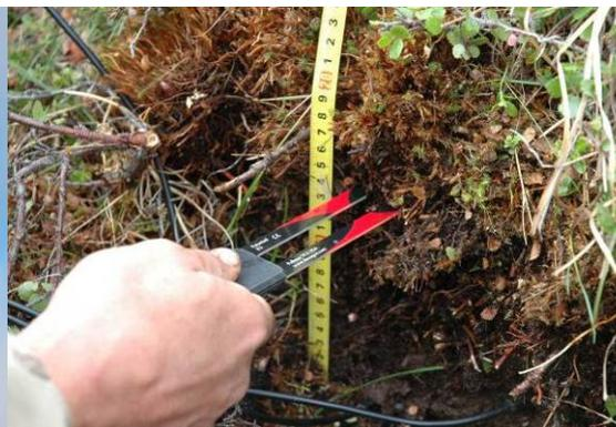
**Fig. 3-6:** Installing soil moisture data loggers at the polygon wall. They were installed shifted against each other with approx. 5 cm height distance between each sensor. We installed the lowest one directly above the permafrost table on July 19<sup>th</sup>.
