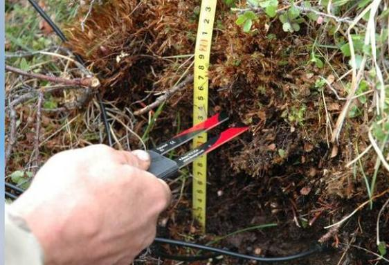
**Fig. 3-6:** Installing soil moisture data loggers at the polygon wall. They were installed shifted against each other with approx. 5 cm height distance between each sensor. We installed the lowest one directly above the permafrost table on July 19<sup>th</sup>.
