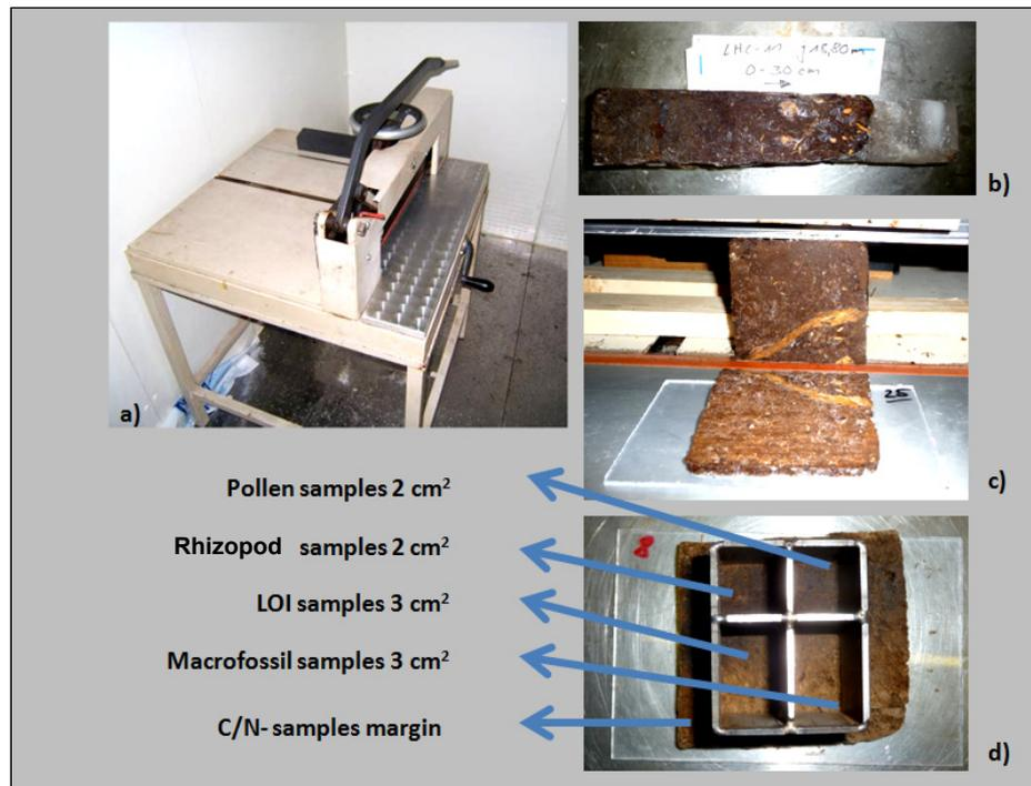
**Fig. 6-10:** Sample preparation for high resolution palaeoecological studies. a) DAMOCLES instrument for peat slice cutting. b) Frozen peat core. c) Peat slice of 0.5 cm. d) Puncher with subsamples.
