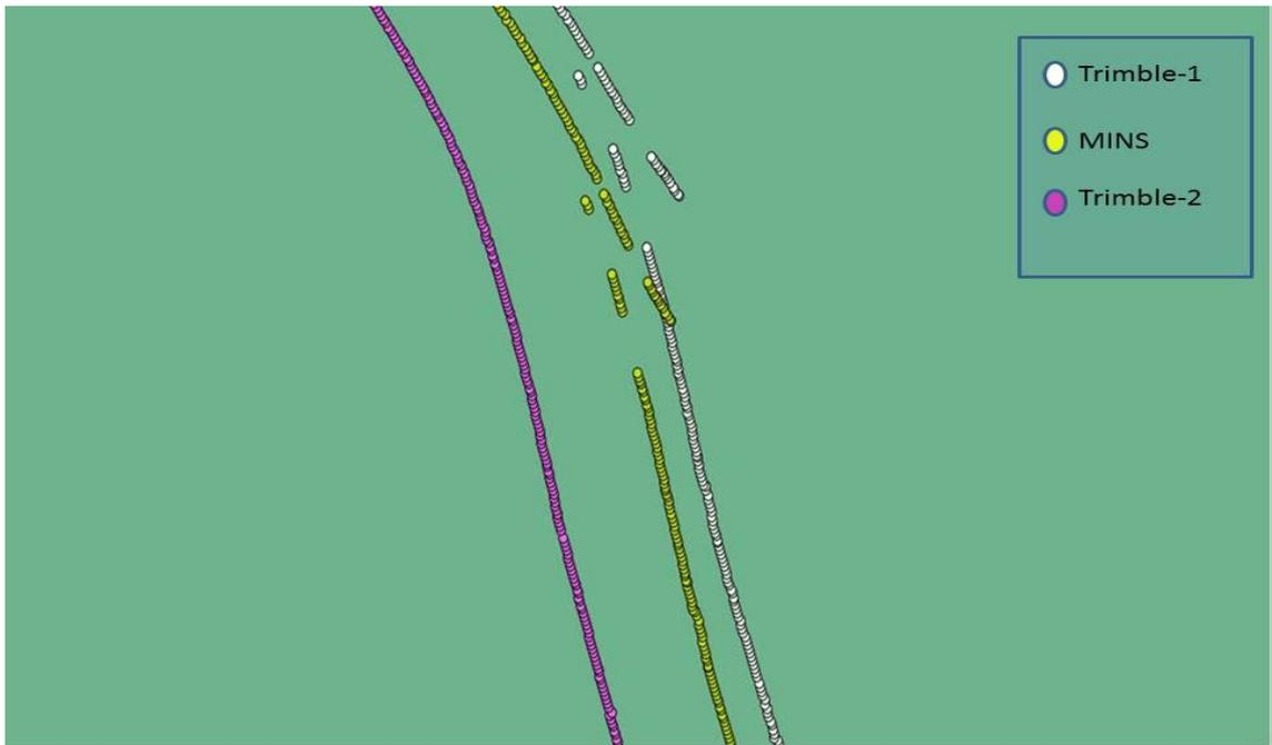
Figure 34: error produced by Trimble antenna and a similar behavior followed by MINS.
