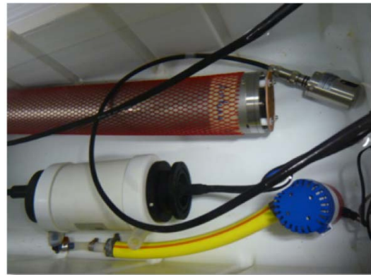
Fig. 6.1: Picture of the in-situ sensors inside the flow-through box (from left to right): HGTD sensor with a connected pump (blue), HydroC™/CO 2 and oxygen optode.
