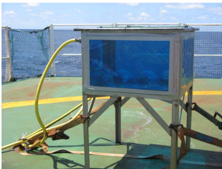
Fig. 11.1: Microcosm for the incubation of bottled water samples used for the assessment of carbon and nitrogen fixation rates. Via the microcom temperature and light- conditions of about 10 m water depth were simulated. Photograph by Tina Baustian
