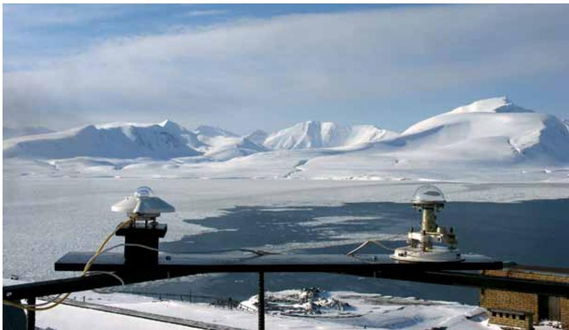
Fig. 2.1-2. Yanishevsky-Savinov (right) and Kipp and Zonen (left) pyranometers used in intercomparisons carried out at the Russian station Barentsburg (Svalbard) in April 2008.
