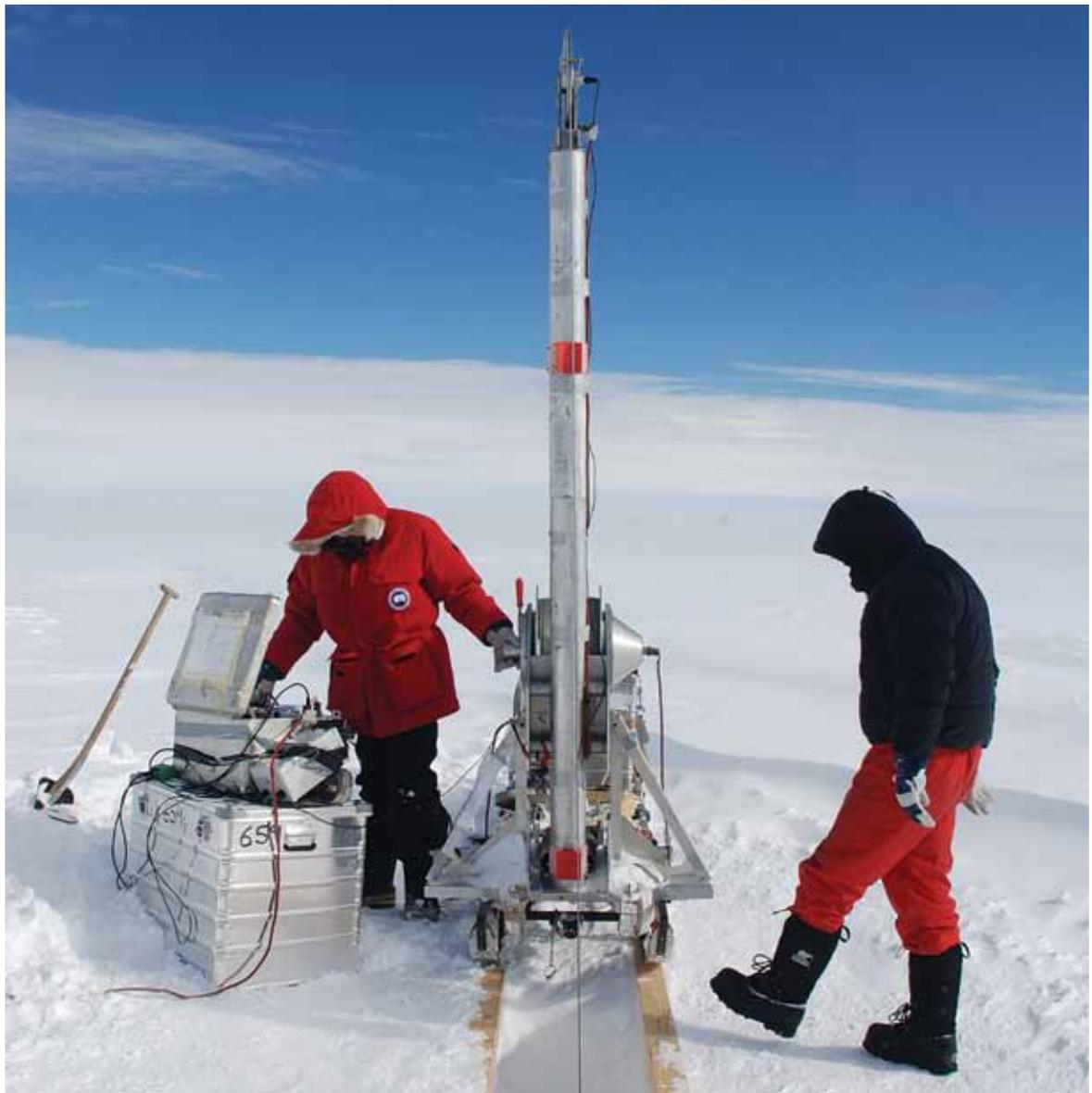
Fig. 2.4-4. Drilling a shallow ice core near the NEEM site on the Greenland Ice Sheet, July 2008.
