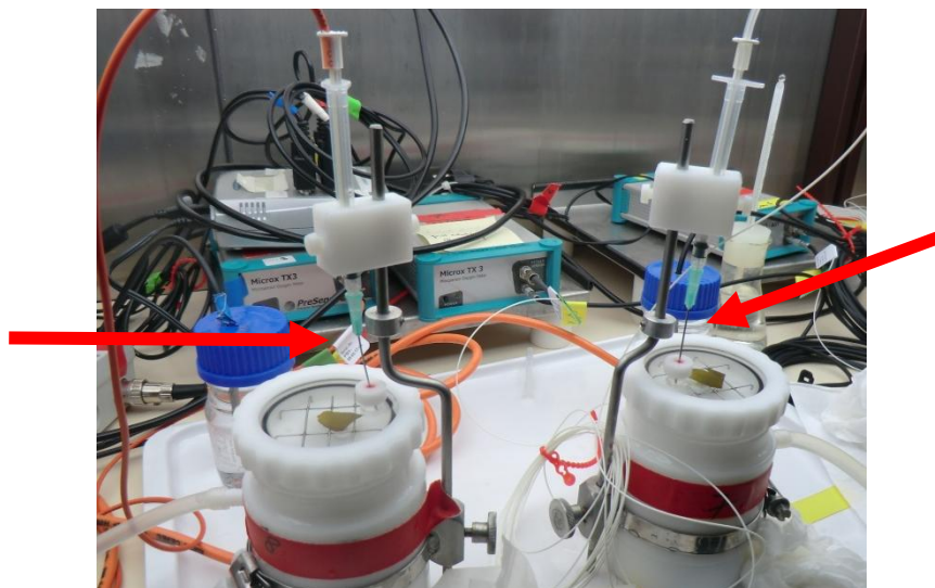
Fig. 6: Experimental set-up for the measurement of photosynthetic activity. Apical tips of Fucus serratus were transferred into the white incubation chambers for 30 minutes (15 minutes each for measurement of respiration and gross photosynthesis). During this time, the oxygen consumption and/or production was measured via a needle type oxygen micro sensor (red arrow).
