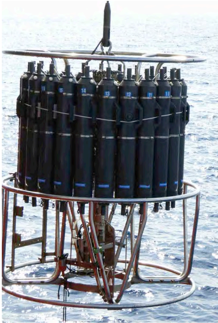
Figure 3-2. The Sea Bird SBE 32 carousel water sampler with the SBE 911 plus CTD profiler.
