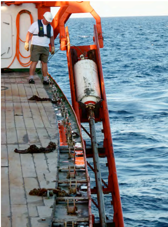
Figure 3-5: Deployment and retrieval of 30 m - Piston Corer
