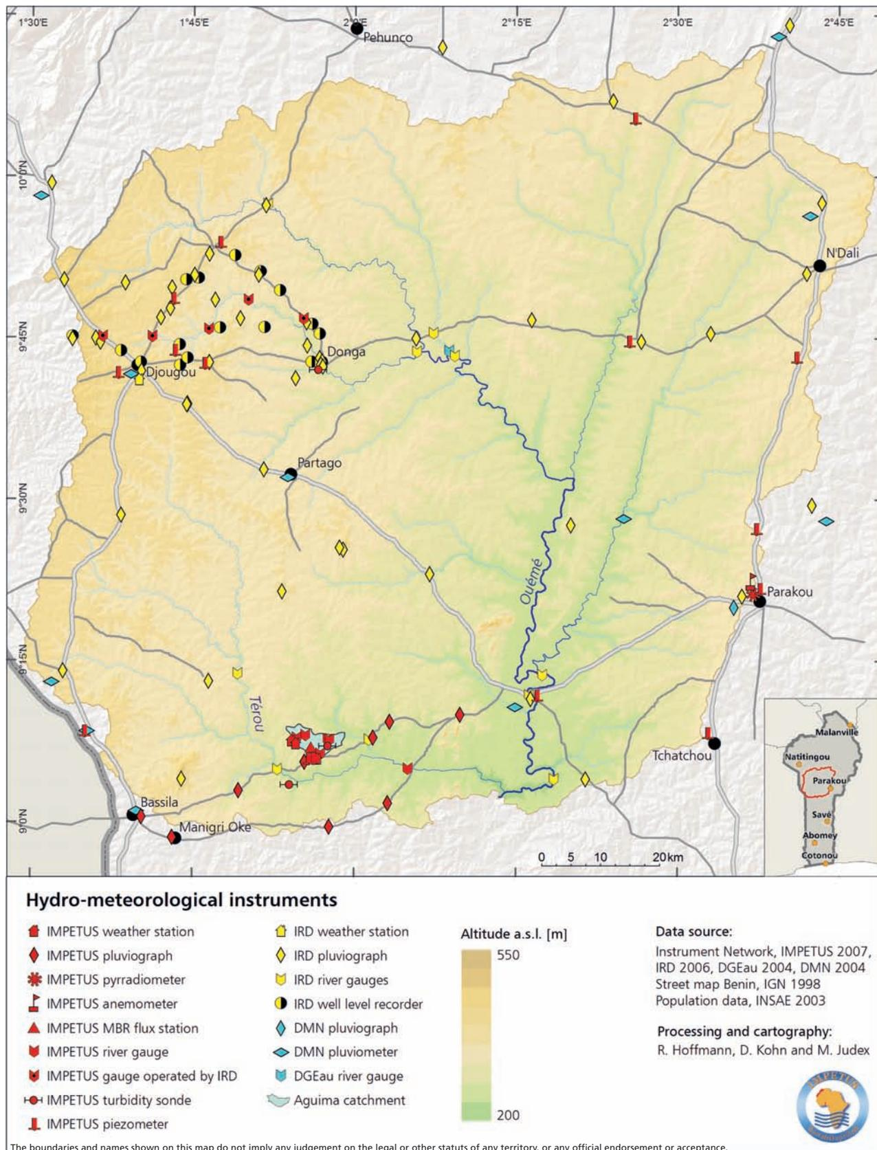
**Fig. 1:** Network of hydro-meteorological instruments in the Upper Ouémé catchment, Benin. Further information regarding the instrumentation network can be found in the Internet: <http://www.impetus.uni-koeln.de> (IMPETUS) and <http://medias.obs-mip.fr/amma> (AMMA-France).
