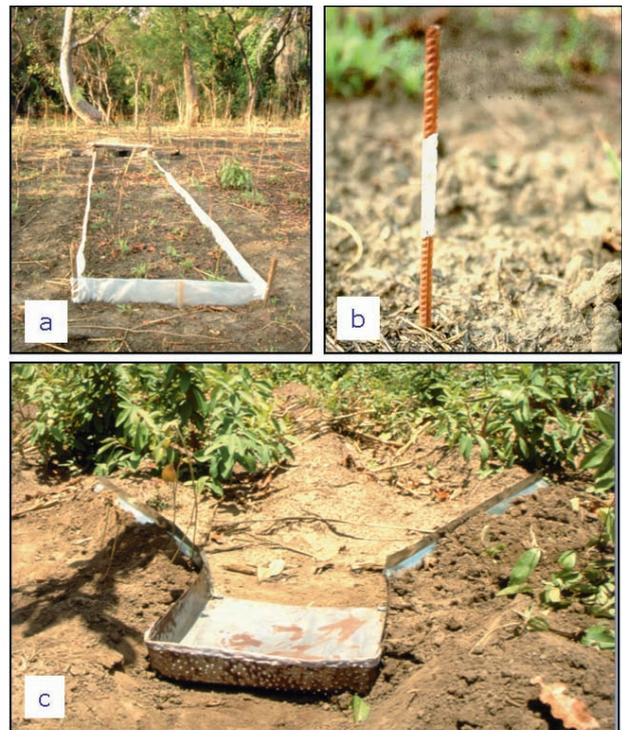
Fig. 1: Erosion plot (a), erosion nail (b) and sediment trap (c)
