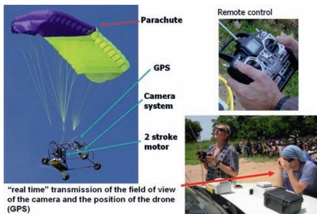
Fig. 1: Elements of the ultra light vehicle.
