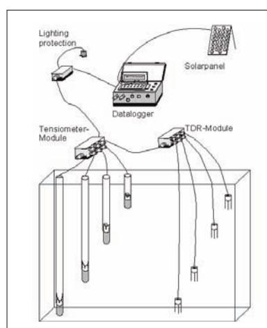
**Fig. 2:** Installation scheme of the soil water measuring plot.
