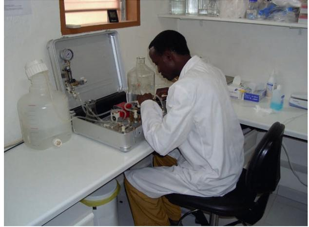
Fig. 2: Sample filtration for viral analysis
