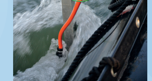
Fig. 3. The AWI RV Christine was used to carry out the seismic surveys. The SES2000 can be seen on the port side of the vessel.
