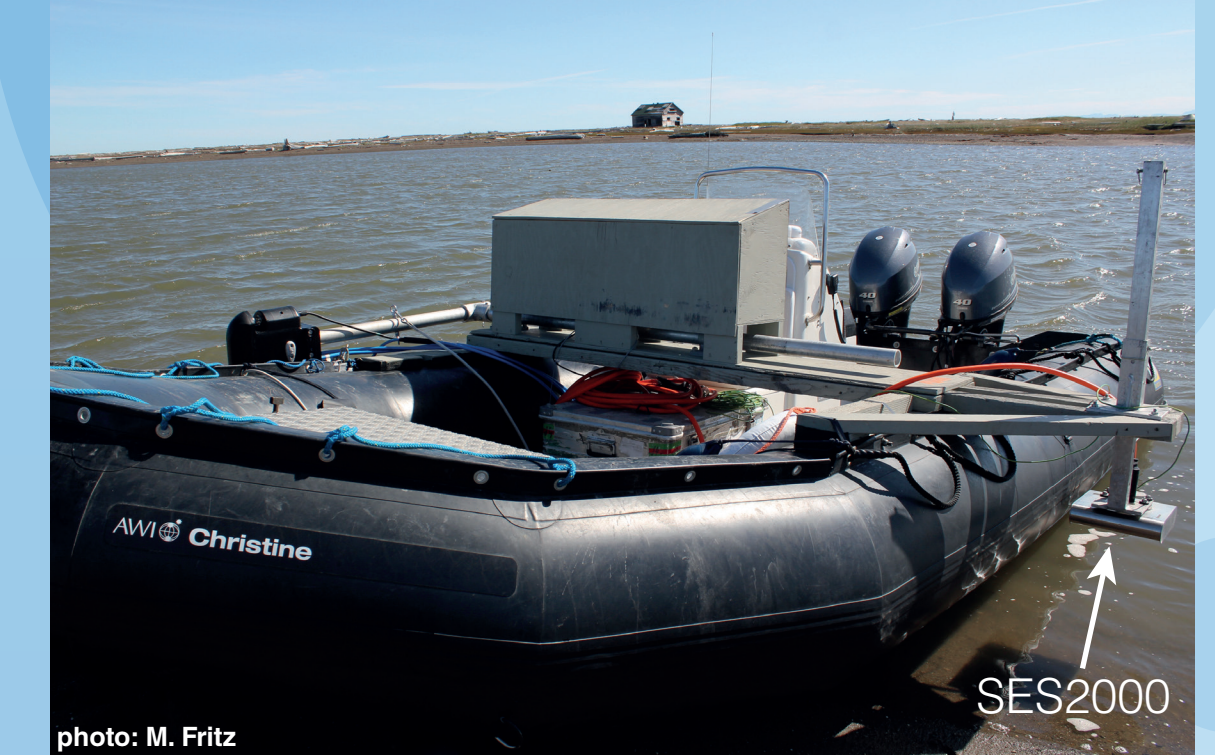
Fig. 3. The AWI RV Christine was used to carry out the seismic surveys. The SES2000 can be seen on the port side of the vessel.
