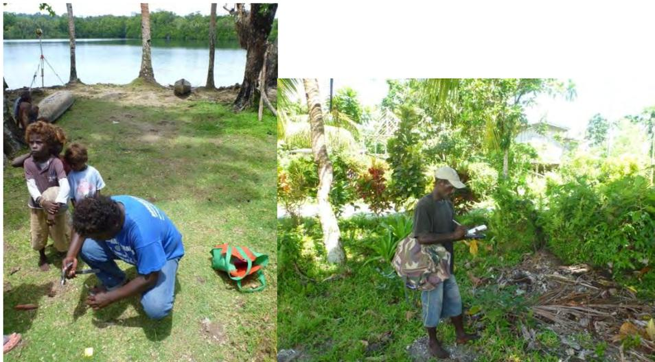
**Figure 30** Marking contours with survey peg (left) and GPS (right)
