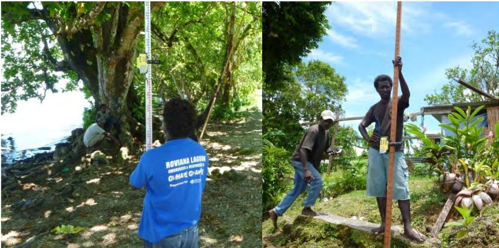
Figure 29 Laser detector attached to 4 m staff (left) and locally created staff (right)
