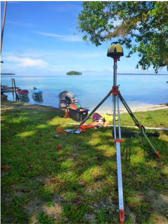
Figure 28 Tripod and laser level set up ready to survey
