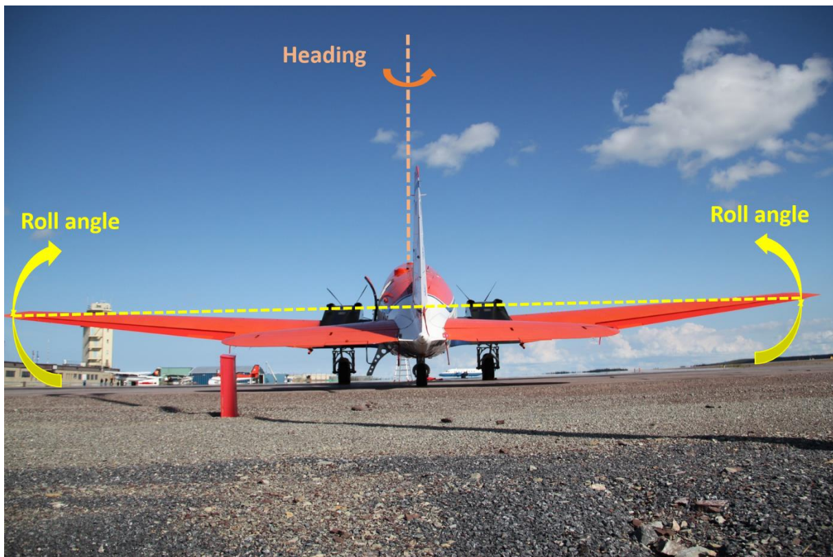
Fig. 7: Illustration of the roll angle and the heading of an airplane. The picture shows Polar 5 at the airport in Inuvik. Picture: K. Kohnert.
