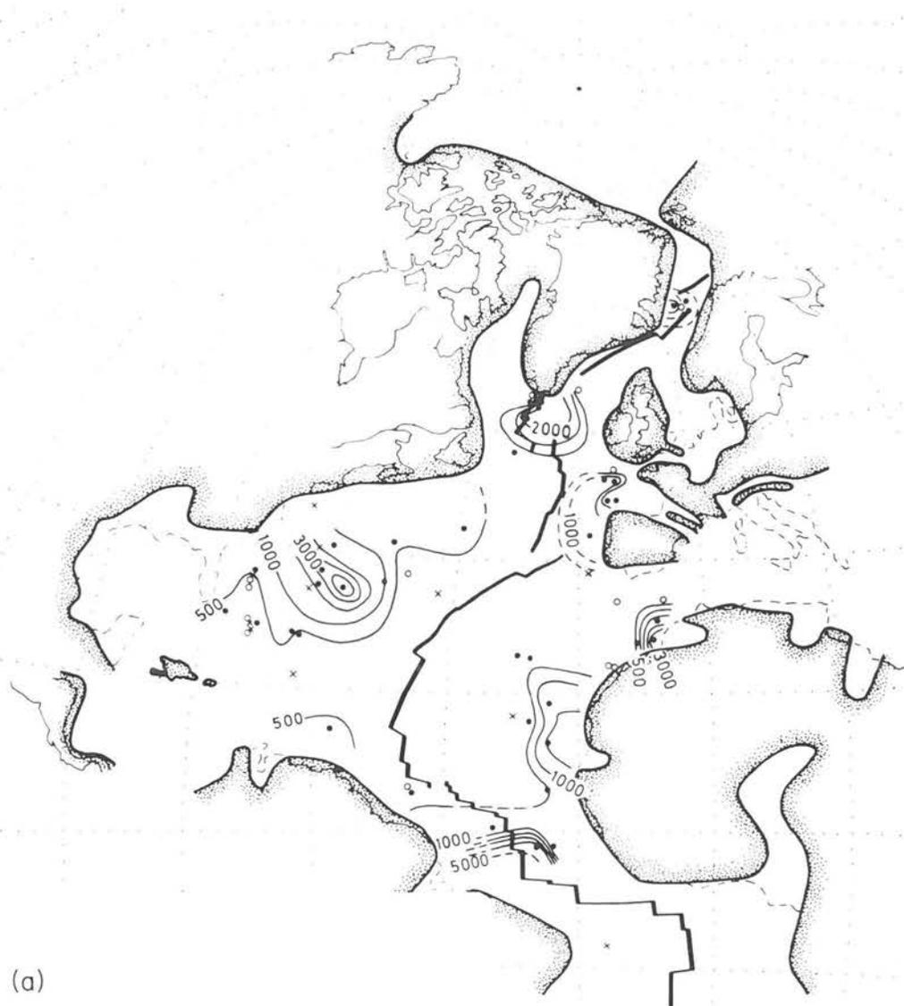
FIG. 4. Accumulation rates of bulk sediment in the North Atlantic in Palaeogene times ( $\text{g cm}^{-2}\text{Ma}^{-1}$ , averaged). The data have been plotted onto palinspastic maps taken from Thiede (1979). DSDP Sites: ● = data; ○ = hiatus; × = no data. (a) 50–46 Ma; (b) 30–26 Ma.
