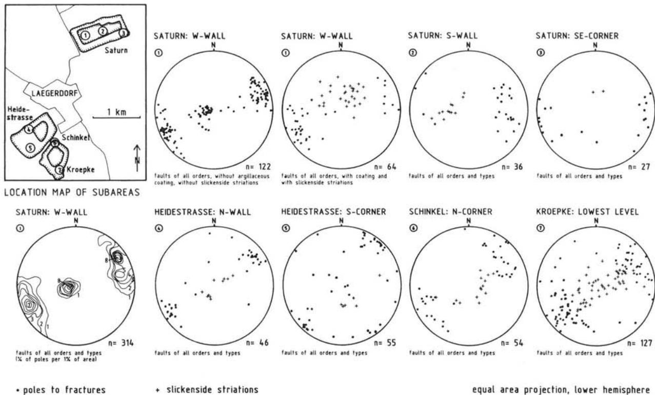
Fig. 3. Stereographic plots as equal area projections of the seven subareas indicated on the index map.
