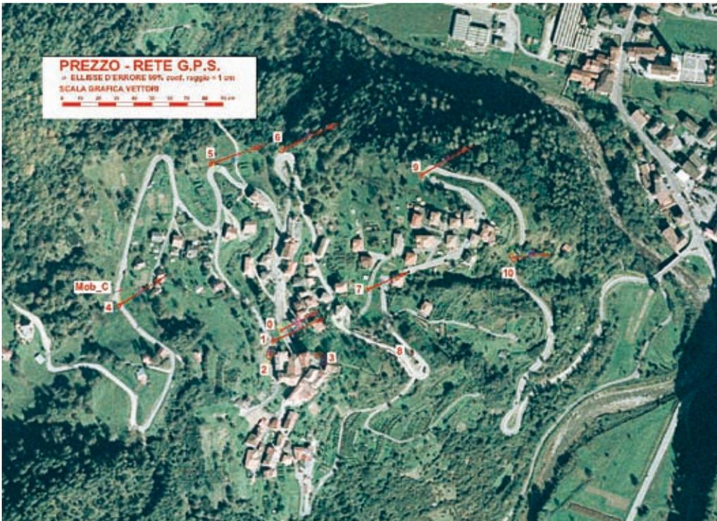
Fig. 5.2.13 - Prezzo landslide; GPS network and displacement vectors.
