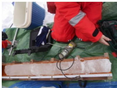
Fig. 1b: Ice drilling core. Direct after sampling the temperature profile is being measured. (foto Jörg Göttlicher).
