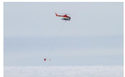
Fig. 6: Ice thickness measurements made over Antarctic sea ice with the EM-Bird (©: Martin Schiller)
