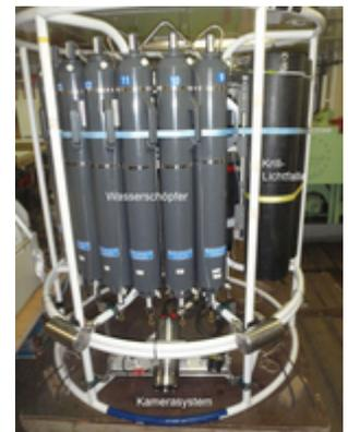
Fig. 2: CTD-Waterrosette with camera system and krill-light trap. (Rob King)
