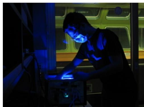
Fig. 4: Atmospheric and sea ice chemistry group: Johannes Zielcke is cleaning and preparing the cavity-enhanced DOAS instrument for measurements of radicals over the sea ice. (Photo Hans-Werner Jacobi).
