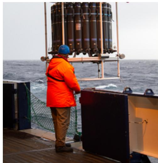
Fig. 3. Water sampler with CTD sensor
