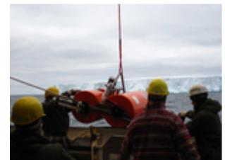
One of the ocean-bottom seismometers (OBS) returned from the seafloor in front of a large iceberg and is lifted back on deck. (photo: K. Gohl)
