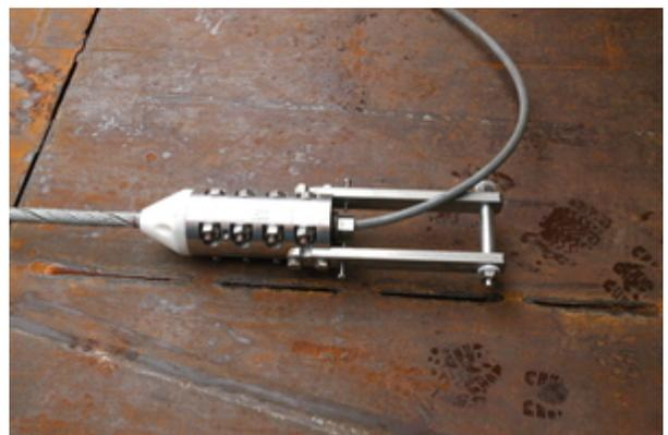
The assembled new cable termination. (photo: E. Dunker)
