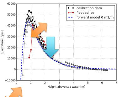
General **offset** to the forward model due to imprecise calibration of individual frequencies.
