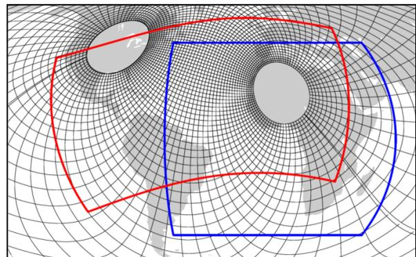
Figure 1. MPI-OM TR04 setup (black lines). REMO-DEP setup (blue line) and REMO-NAT setup (red line). Every 12th grid line is shown.
