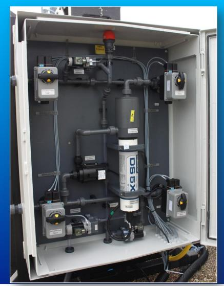
One system for two mesocosms: Hydrolab DS5X parameters measured at the moment
