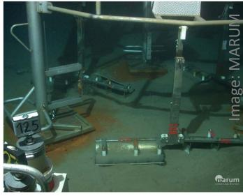
ROV- (& crawler-) manipulated biogeochemical measurement systems | MPI
