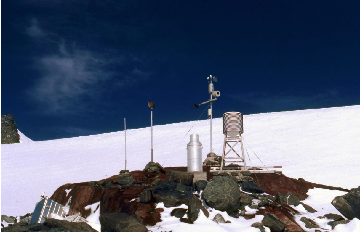
'Gletschermitte' station (1985) with Belfort precipitation gauge, the wind recorder according to Woelfle on top of the mast, the Stevenson screen containing the thermo-hydrograph and the minimum-maximum-thermometers. At the end of the horizontal beam the protective case with the camera is mounted. (Photo: M. Weber)
